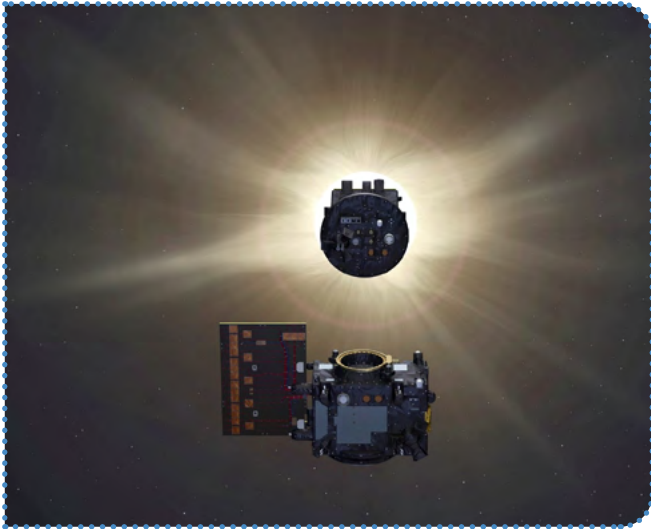
Proba-3 Occulter spacecraft eclipsing the Sun for the Coronagraph spacecraft. Credit: © ESA – P. Carril
