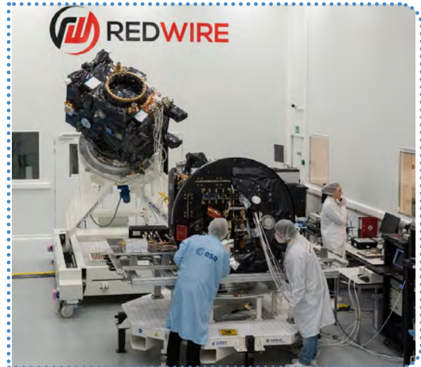
Proba-3's Occulter seen in the foreground, and Coronagraph spacecraft, during pre-flight testing at Redwire in Belgium in spring 2024. Credit: © ESA – P. Sebirot
