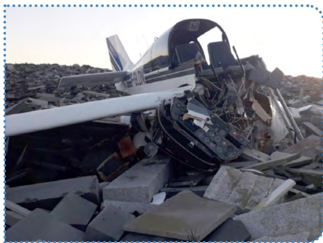
Figure 3: Wreckage of a DR400 after a collision with a ULM on approach to Lunéville-Croismare Airport in France. The collision without fatal injuries was due to the use of different radio frequencies. Source: Police de Lunéville
