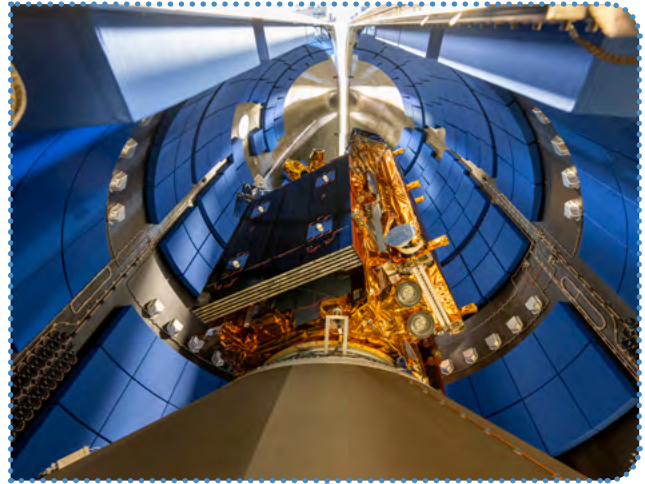
Figure 3 Sentinel-1D encapsulation (credits: ESA - M. Pédoussaut)
