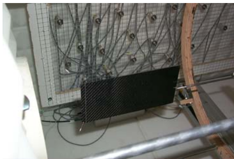
Figure 7.4 Experimental set-up for measurements of trailing-edge noise of a thin flat plate (AWD).
