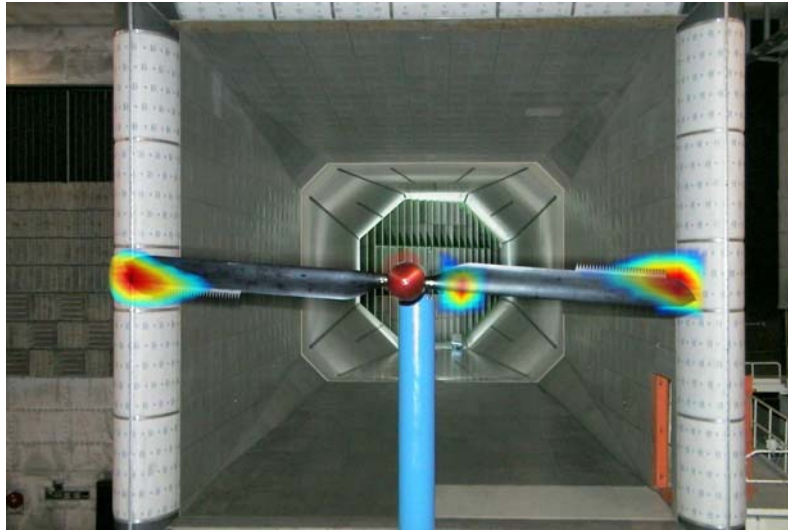
Figure 7.2 Acoustic image of model wind turbine at 8000 Hz, obtained with ROSI.
