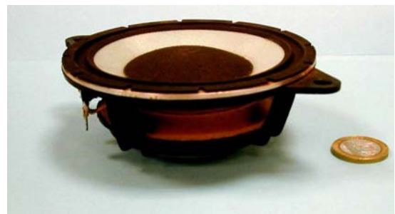
Example of new actuator for ANC (Electrodynamic direct radiator of CTTM).
