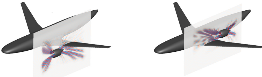
Fig. 1. Instantaneous pressure fluctuations with one-sided engine aircraft in the vertical nacelle mid-section plane: UWN configuration (a.); OWN configuration (b.).
