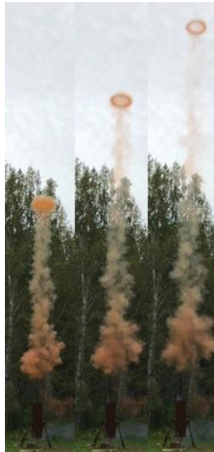
Fig. 35. High speed camera diagnostics of vertical movement of the vortex ring, duct diameter 80 cm.
