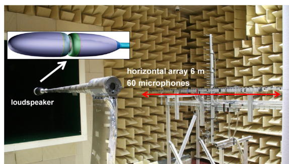
Fig. 22. Horizontal microphone array and aerodynamically covered loudspeaker in the DNW-NWB open test section.
