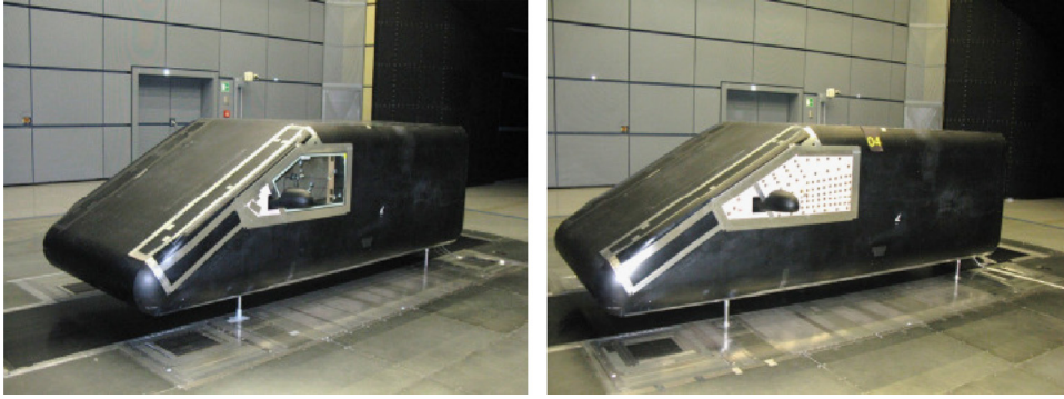
Fig. 29. Wind-tunnel test: glass module (left), sensor module (right) [29].
