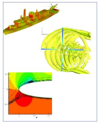
Figure 2: Some examples of emerging CFD computations From right to left: helicopter landing on a ship, rotor in bladevortex-interaction state, transitional flow near the leading edge of a rotor blade.
