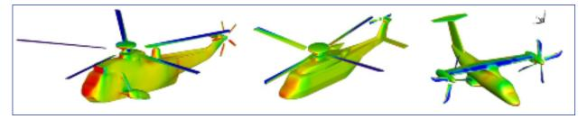
Figure 1: Examples of CFD computations around rotorcraft configurations at trimmed flight.
