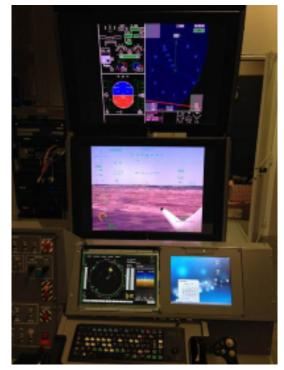
Inside the GCS (Ground Control Station) for the MIDCAS UAV demonstrator. (EDA)
