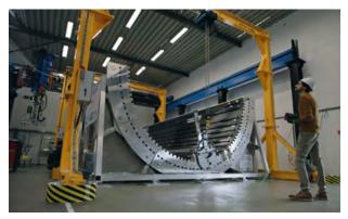
Figure 7: An automated manufactured lower shell of the fuselage of the future (Credits: Oculus Film)
