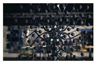
Figure 3: An acoustic camera for noise measurements (Credits: Oculus Film)
