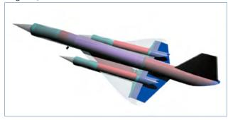
Figure 3 – M3 Configuration with fuselage and wing skins off. Cyan air flow path, blue wing nozzle and thrust surfaces red fuel tanks, magenta cabin
