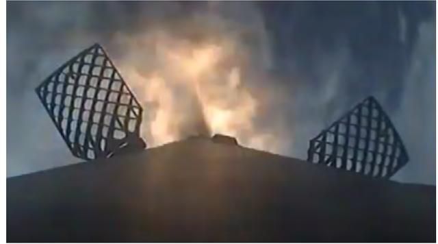
Figure 6: Demo-2 SpaceX Falcon 9 rocket booster during its re-entry burn a few minutes after launch – Image credit: NASA TV
