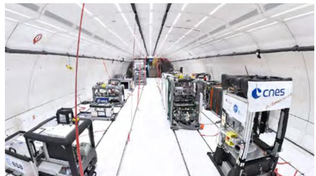
Figure 2: In the cabin of the Airbus A310 Zero G aircraft, all seats were removed along the 20 meters long front part of the cabin, thus providing the largest ZERO G aircraft experimental area in the world.
