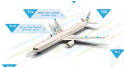
ACTIVE FLOW SEPARATION CONTROL AT THE OUTER WING
