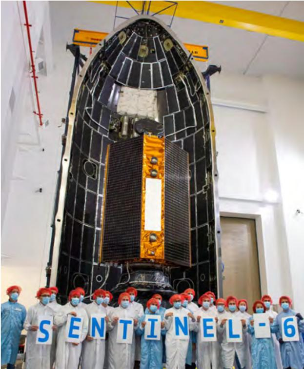
Inside SpaceX's Payload Processing Facility at Vandenberg US Air Force Base (CAL), the US-European Sentinel-6A Michael Freilich is being encapsulated in the SpaceX Falcon 9 payload fairing, 3 November 2020. © Credit NASA
